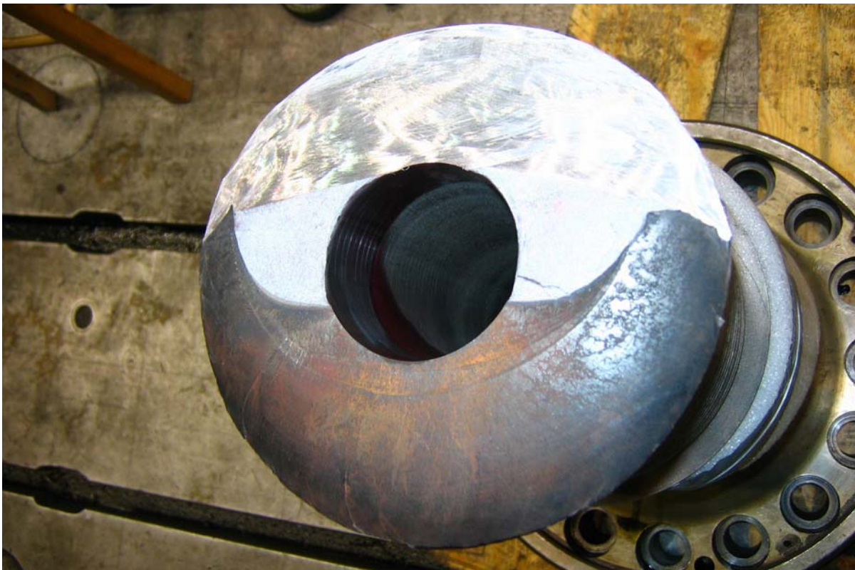
Figure 2. The crack was opened after being ground down at 12 o'clock and subsequent brittle fracture. The smooth fracture features indicate a fatigue failure with the origin at about 6 o'clock.
